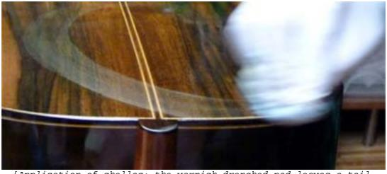
[Application of shellac: the varnish drenched pad leaves a tail that makes a new layer in the thickness of few molecules.]
